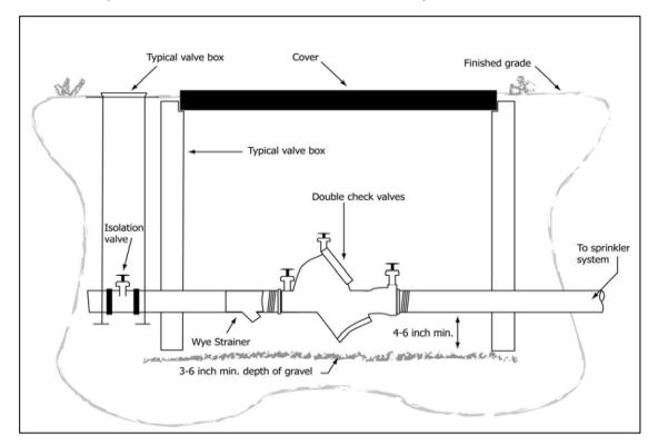
The double check backflow prevention device must be tested upon installation before the system is put into service by a licensed tester that is registered with the City of Arlington Water Resources (WR) Department. The results of the Backflow Prevention Assembly Test (BPAT) must be recorded on forms provided by WR. The BPAT test results shall be provided to the irrigation inspector when the installation of the double check backflow prevention device is inspected.
